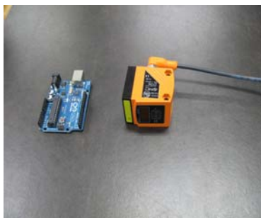
Figure 7 Arduino and PIR sensor
