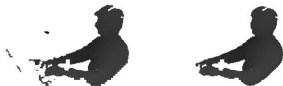
Figure 4. The left image is the raw depth silhouette captured by the Kinect, and the right image is the same image after going through our noise reduction.
