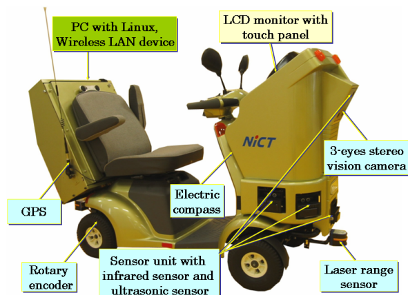
図 1: Low-speed outdoor mobile vehicle with stereo vision camera
