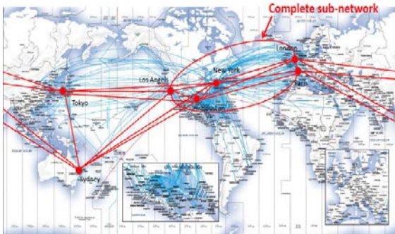
Fig.4. Example of global airline network based on the multi-star small-world network ( n=7 ).
